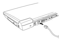
Figure 4-12 Connecting the LAN cable
